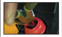
**Step 5:** When installed correctly, the TEZOM seal and secondary seal sit flush against each other and level against the exhaust chamber.
