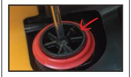
**Step 4:** Using needle nose pliers to grab only the guide(making sure not to damage the sealing surface) and press until the guides locking tabs fully engage with the slot. Repeat until all 3 guide have been installed.
