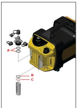
Carefully remove old o-rings. Step 1: DO NOT use sharp tools, this can damage the o-ring grooves.
