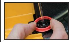
**Step 3:** Install the new TEZOM seal(D) making sure each guide engages with a (triangle-shaped) slot.
