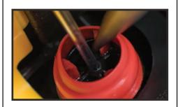
**Step 2:** Install the new TEZOM secondary seal(E) Push until flush and level with the exhaust chamber.
